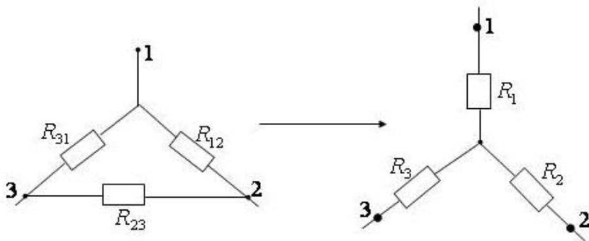
$R_1 = \frac{R_{12} \cdot R_{31}}{R_{12} + R_{23} + R_{31}} \quad R_2 = \frac{R_{12} \cdot R_{23}}{R_{12} + R_{23} + R_{31}} \quad R_3 = \frac{R_{23} \cdot R_{31}}{R_{12} + R_{23} + R_{31}}$
