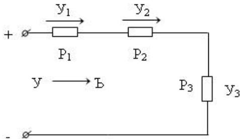
$$P = C^2(R_1 + R_2 + R_3) = C(U_1 + U_2 + U_3)$$
