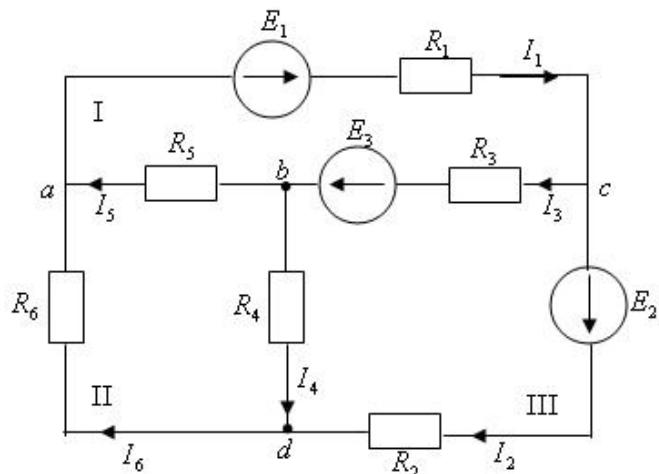
$$\text{Q} - I_4 + I_5 = 0 \quad I_1 R_1 + I_3 R_3 + I_5 R_5 = E_1 + E_3$$
