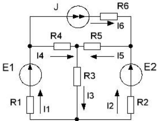
$\text{Q}_6 R_6 + I_5 R_5 - I_4 R_4 = JR_6$
