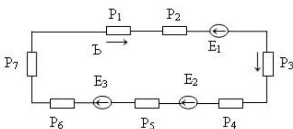
$\text{Q}_1 + E_2 = J(R_1 + R_2 + R_5 + R_6)$
