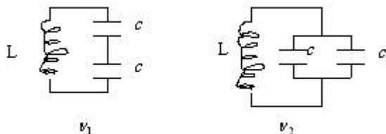
$v_1 = 2v_2$
