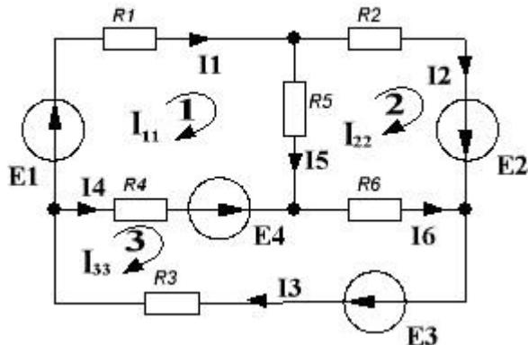
$Q_{11}(R_1 + R_5 + R_6) - I_{22}R_5 - I_{33}R_2 = E_1 - E_2$
