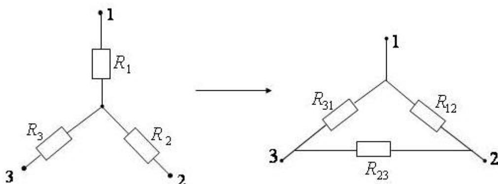
$R_{12} = \frac{R_1}{R_2} + \frac{R_3}{R_2} + R_{13} \quad R_{23} = \frac{R_1}{R_3} + \frac{R_2}{R_3} \quad R_{31} = \frac{R_2}{R_1} + \frac{R_3}{R_1}$
