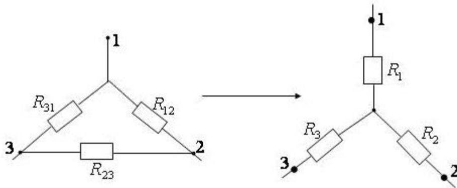
$R_1 = \frac{R_{12} \cdot R_{23}}{R_{12} + R_{23} + R_{31}}$     $R_2 = \frac{R_{31} \cdot R_{23}}{R_{12} + R_{23} + R_{31}}$     $R_3 = \frac{R_{23} \cdot R_{12}}{R_{12} + R_{23} + R_{31}}$
