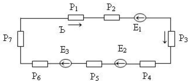
$$Q_1 + E_2 = J(R_1 + R_2 + R_5 + R_6)$$
