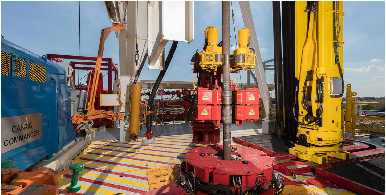
Fig. 1.4 Robotic pipe handling system. ( https://www.nabors.com )
