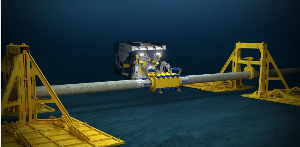
Fig. 1.9 Deepwater Pipeline Repair System. ( https://www.oceaneering.com )
