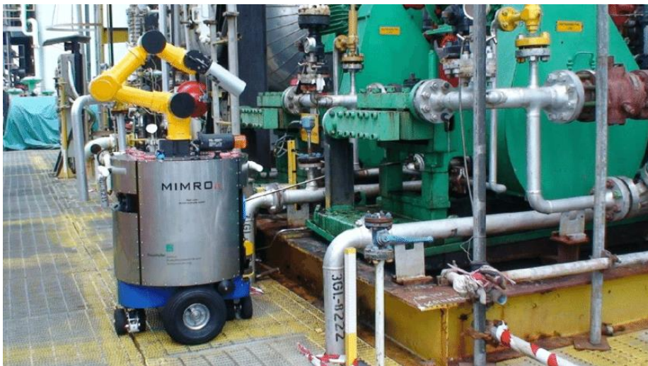
Fig. 1.11 The Fraunhofer Inspection Robot. ( https://www.researchgate.net )
