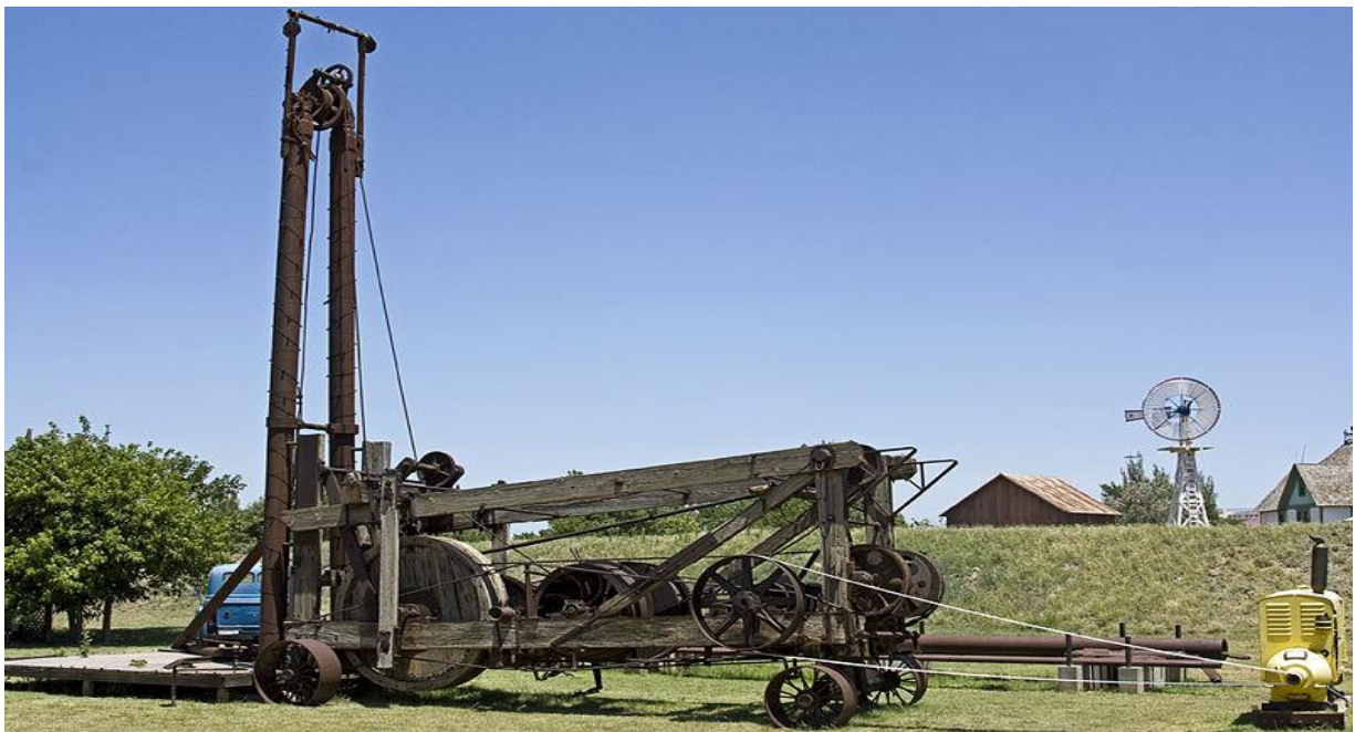
Fig. 1.1 Cable drilling rig. ( http://www.ritchiewiki.com )
