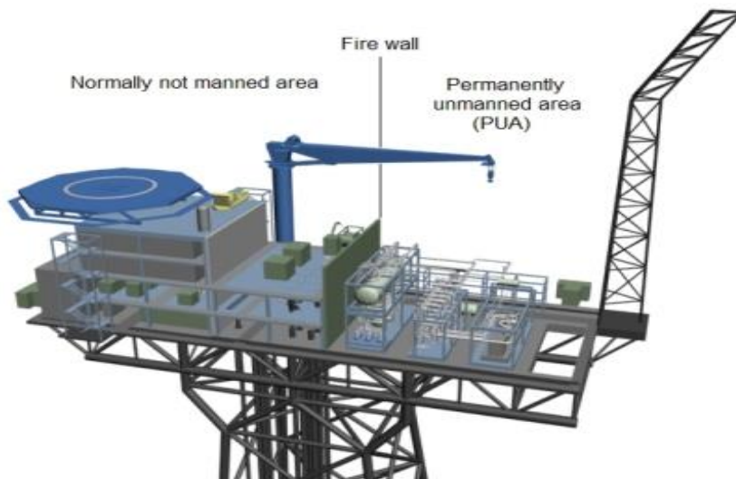
Fig. 1.10 SINTEF Topside Remote Platform. ( https://www.sintef.no )
