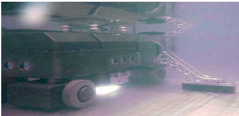
Fig. 1.15 In-Tank Inspection Robot. ( http://www.newtonlabs.com )
