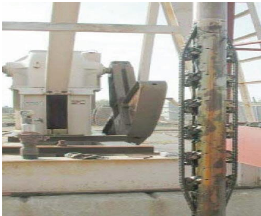
Fig. 1.7 MicroRig robotic intervention tool by iRobot.
