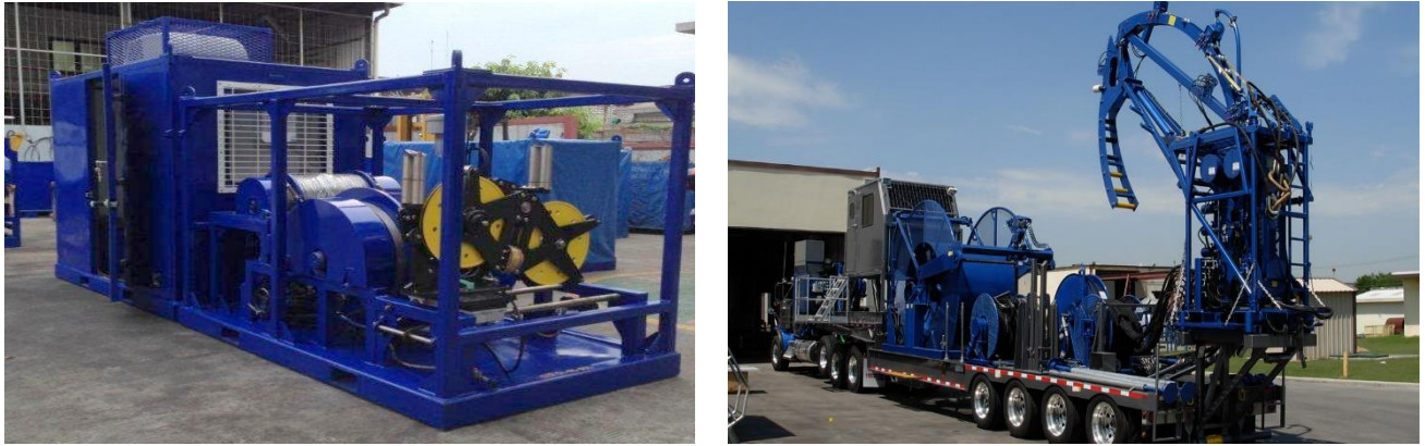
Fig. 1.5 Slickline unit and coiled tubing unit. ( http://prowell-energy.com )
