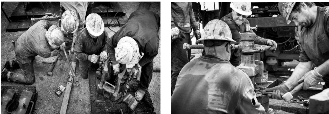
Fig. 1.3 The two rig hands on left tend to the wellhead while the others prepare the slips (coupling that holds the pipe in place) for the 2 3/8-inch pipe. Image © Chad Ziemendorf. ( http://www.intersectionjournal.com )
