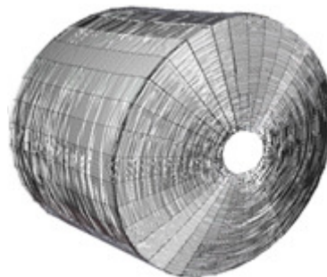
Figure. 4. A three-dimensional package model from Rieter R-40 pneumomechanical machine
