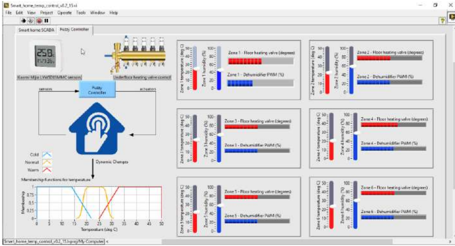
Figure 10. Fuzzy Logic Smart Energy Control - Setup
