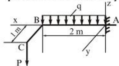
$Q_A = 25 \text{ kN}, M_x = 5 \text{ kN} \cdot \text{m}, M_y = 30 \text{ kN} \cdot \text{m}$
