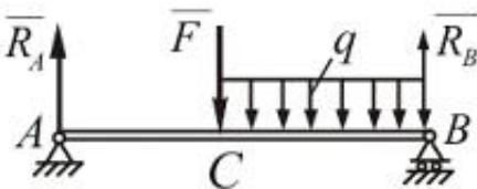
$R_A = 16 \text{ kN}; R_B = 20 \text{ kN}$
