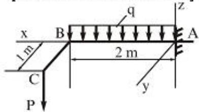
$\Omega_A = 25 \text{ kN}, M_x = 5 \text{ kN} \cdot \text{m}, M_y = 30 \text{ kN} \cdot \text{m}$
