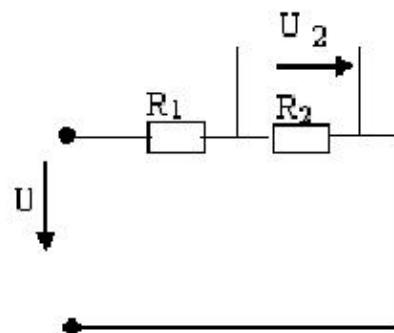
**Дано:**  $R_1 = 30 \Omega$ ,  $R_2 = 20 \Omega$ ,  $U = 125 \text{ V}$ .  $U_2 = ?$
