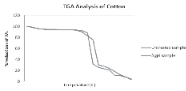
Figure 2: Effect of temperature on weight reduction of cotton fabric
